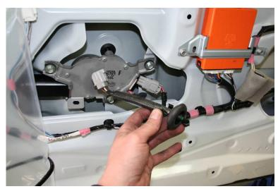
3. Plug in short camera loom into original plug
