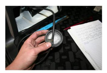
7. Fit 30mm grommet supplied into hole in door.
