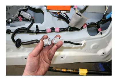
4. Remove jack from storage area, and make a small cut in either end of original rubber condute. Feed camera loom through as per photo.
